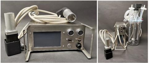
*Cilix are designed to drive independently two Brush-Less-Direct-Current (BLDC) servo motors. Mix as needed for drive of two SUBs, SUF, SUMs. Shown with ID30 adaptor.*
