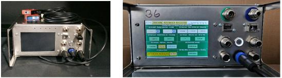
*Clotho-2 is small and compact fitting all electronics for the two channels inside Hephaestus U2 Stainless Steel cabinet. Even with the 5" touch sensitive display.*
